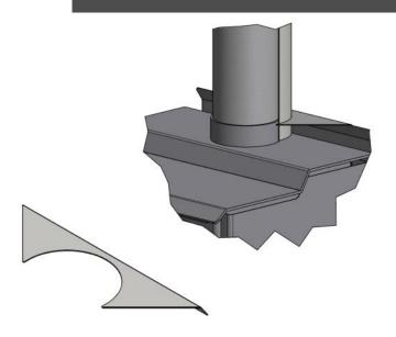
The rear deflector is used for reducing rear clearances for applicable fires (see page 4 for details). It is located loose in the firebox.
