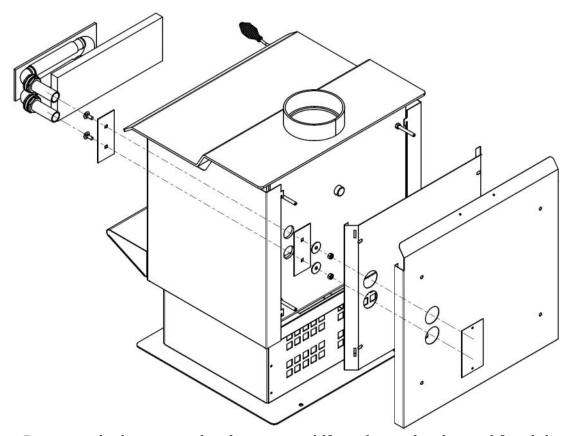
Note: Rear panels do not need to be removed if a tube socket is used for tightening
